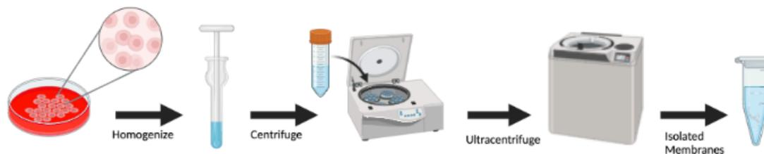
Figure 13: Membrane preparation workflow.
