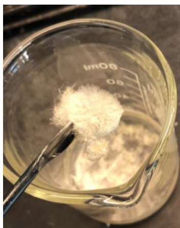
Figure 4. Recrystallized azaxanthone from ethanol produced spidery yellow-white needles.
