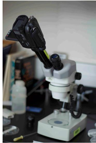
**Figure 13.** Sony Handycam HDR-HC9 camcorder mounted to a dissecting microscope
